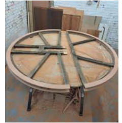
A bell wheel being restored in Trevor's workshop
